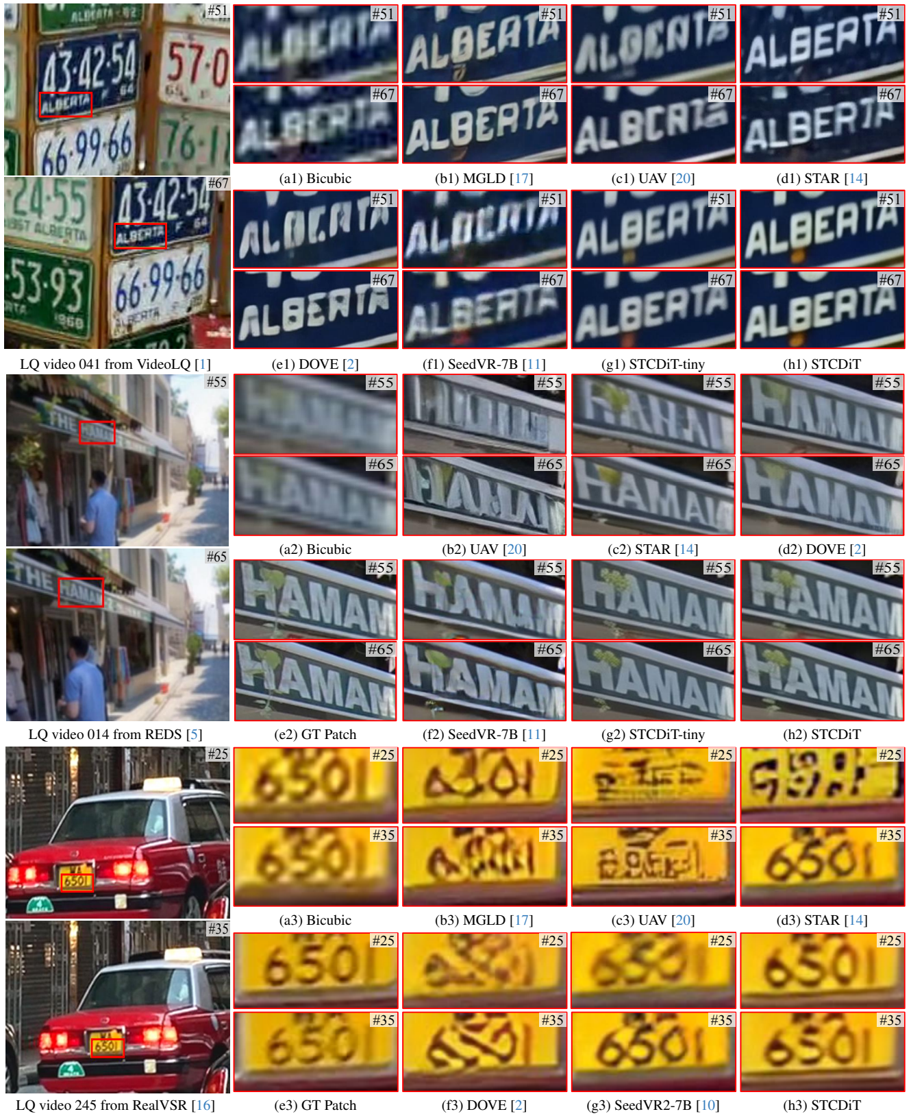
Figure 11. The first and second rows show VSR results ( \times 4 ) on the real-world benchmark [1] and the synthetic benchmark [5], respectively, while the third row shows VSR results ( \times 1 ) on the real-world benchmark [16]. Compared to competing methods, our method restores videos with better temporal consistency and structural fidelity.
