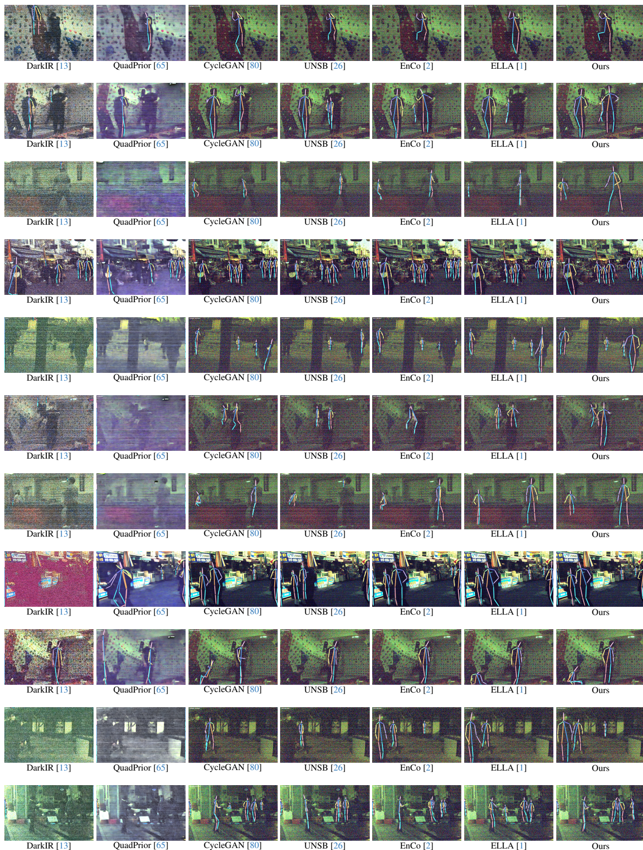
Figure 9. Pose predictions of UDAPose compared against competing methods. The first two columns show results from enhancement-based methods; all other columns display results on the original low-light images. The low-light images are scaled for visualization only.
