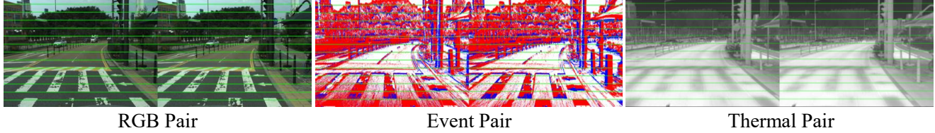
Figure 7. Example of stereo rectification results for the RGB, event, and thermal modalities. The green horizontal lines visualize the epipolar lines, which become well aligned after calibration.
