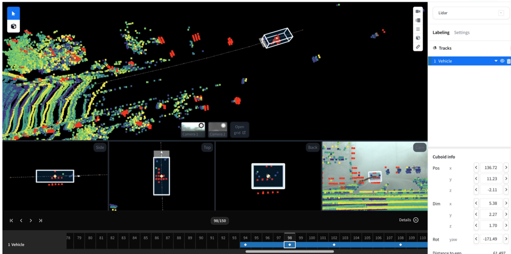
Figure 8. Multi-modal annotation tool. 4D Radar points are shown in red, and LiDAR points are color-coded by timestamp using a viridis colormap. 3D sensor data and 3D annotations can be projected onto camera sensor images, ensuring consistent annotations across modalities under diverse driving conditions..
