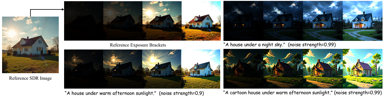
Figure 8. Reference-based HDR exposure brackets generation from an SDR image. Starting from a display-referred SDR image (left), we apply a gamma correction to approximate its linear domain representation and synthesize a set of pseudo-linear reference exposure brackets (middle-top). Although these brackets have limited dynamic range, they serve as structural and exposure-aware guidance. Using an SDEdit [9] noise–denoise process, we progressively inject noise into the reference brackets and perform conditional denoising to generate HDR exposure brackets with enriched dynamic range (middle-bottom). By adjusting the noise strength during SDEdit, we can control the trade-off between fidelity to the reference exposure structure and the generation of plausible high-dynamic-range content (right). This enables reference-guided HDR bracket generation while preserving semantic consistency.
