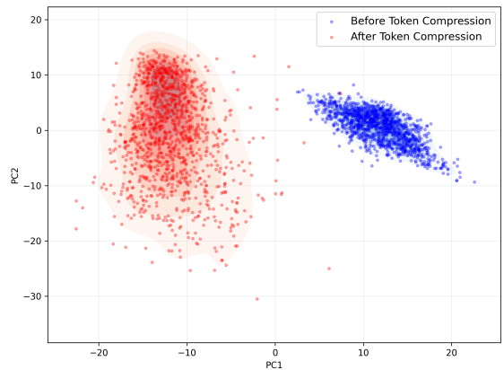
Fig. 3. Impact of visual token compression on visual token embedding. The points represent the coordinates of visual token features after PCA dimensionality reduction, with the kernel density estimation overlaid.
