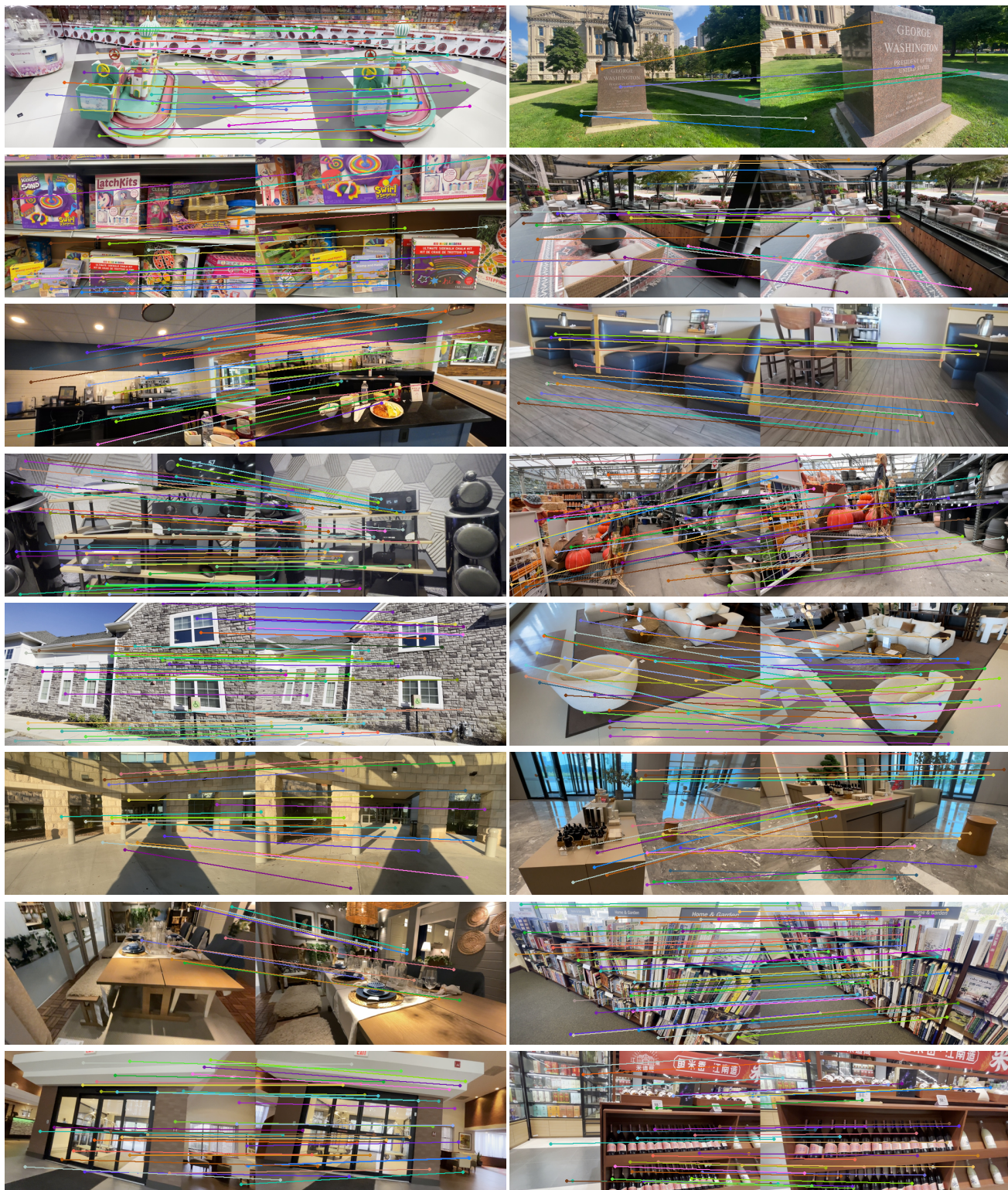
Figure 5. Visualization of Matching on DL3DV. Given query points in the left image, we visualize the matched pixels in the right image. Our matching is robust to large changes in camera viewpoint.
