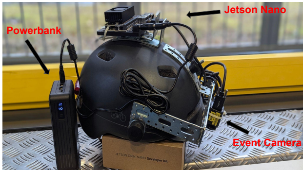
Figure 7. Our head-mounted device setup. The device uses a single fisheye egocentric event camera for input, NVIDIA Jetson Orin Nano for onboard processing, and a portable powerbank for standalone operation.
