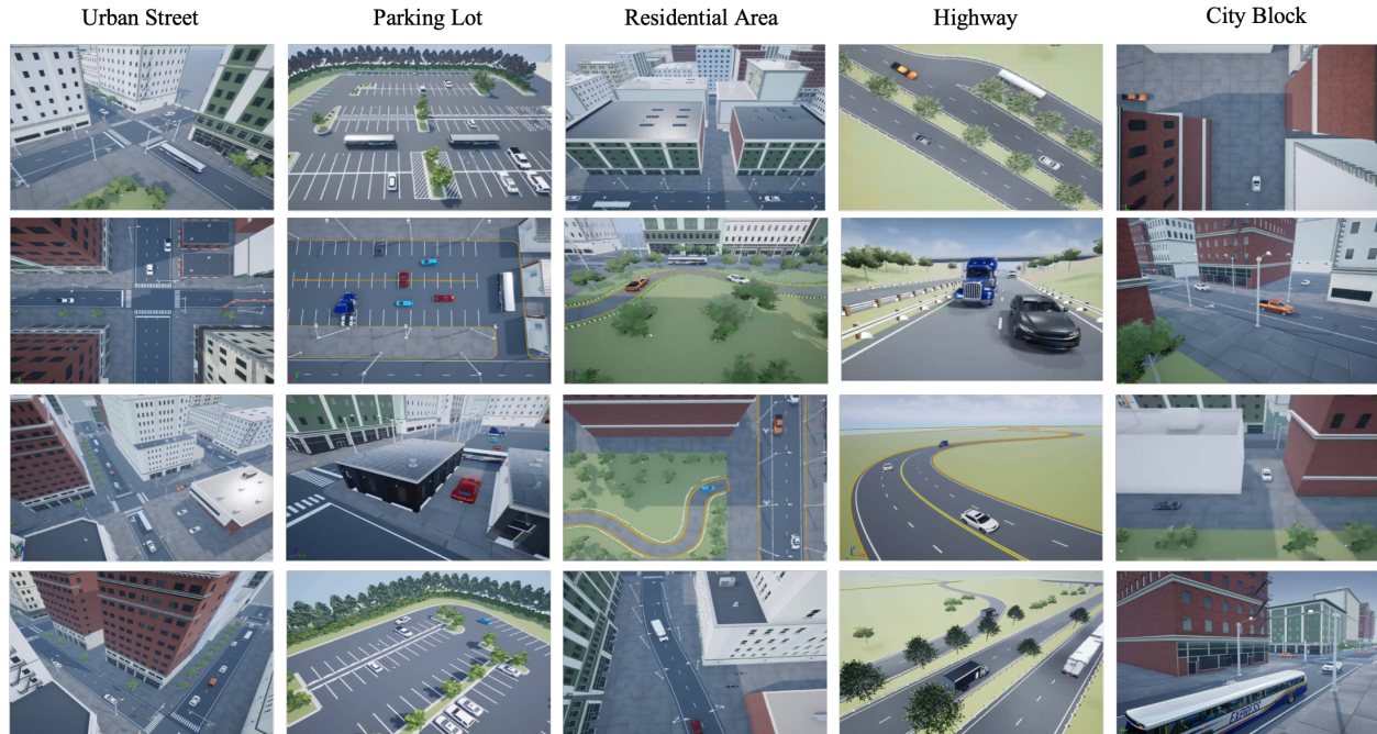
Figure 4. Synthetic NLOS Dataset Scene Types. The scenes cover diverse urban layouts (streets, parking lots, residential blocks) with varied relay interfaces (building facades, walls, vegetation) and hidden objects including cars, trucks, buses, and bicycles.
