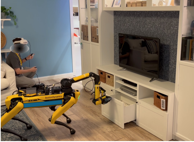
Supplementary Figure 6. Spot Teleoperation The Spot Robot is teleoperated using a Meta Quest 3. We retarget the remote’s 6-DoF pose to the gripper and control the base using the remote mounted Joystick.
