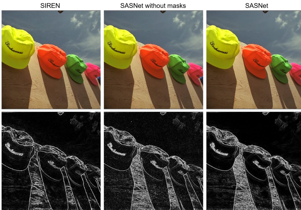
Figure 8. Visual comparison between SIREN, SASNet without masks, and full SASNet. First row shows the image reconstructed and the second row shows the corresponding gradient intensity obtained by network automatic differentiation ( autograd in PyTorch).
