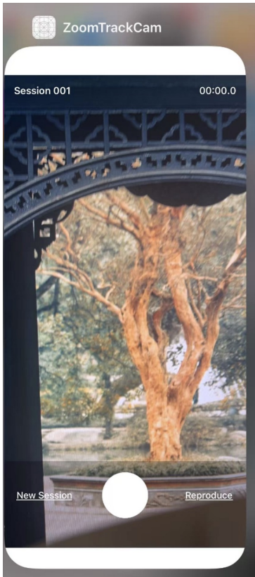
Figure 10. Data capture software. Our app records aligned video pairs by locking exposure and focus, matching file names and durations, enabling reliable Bluetooth triggering for stable control, and using a tripod to remove camera shake.
