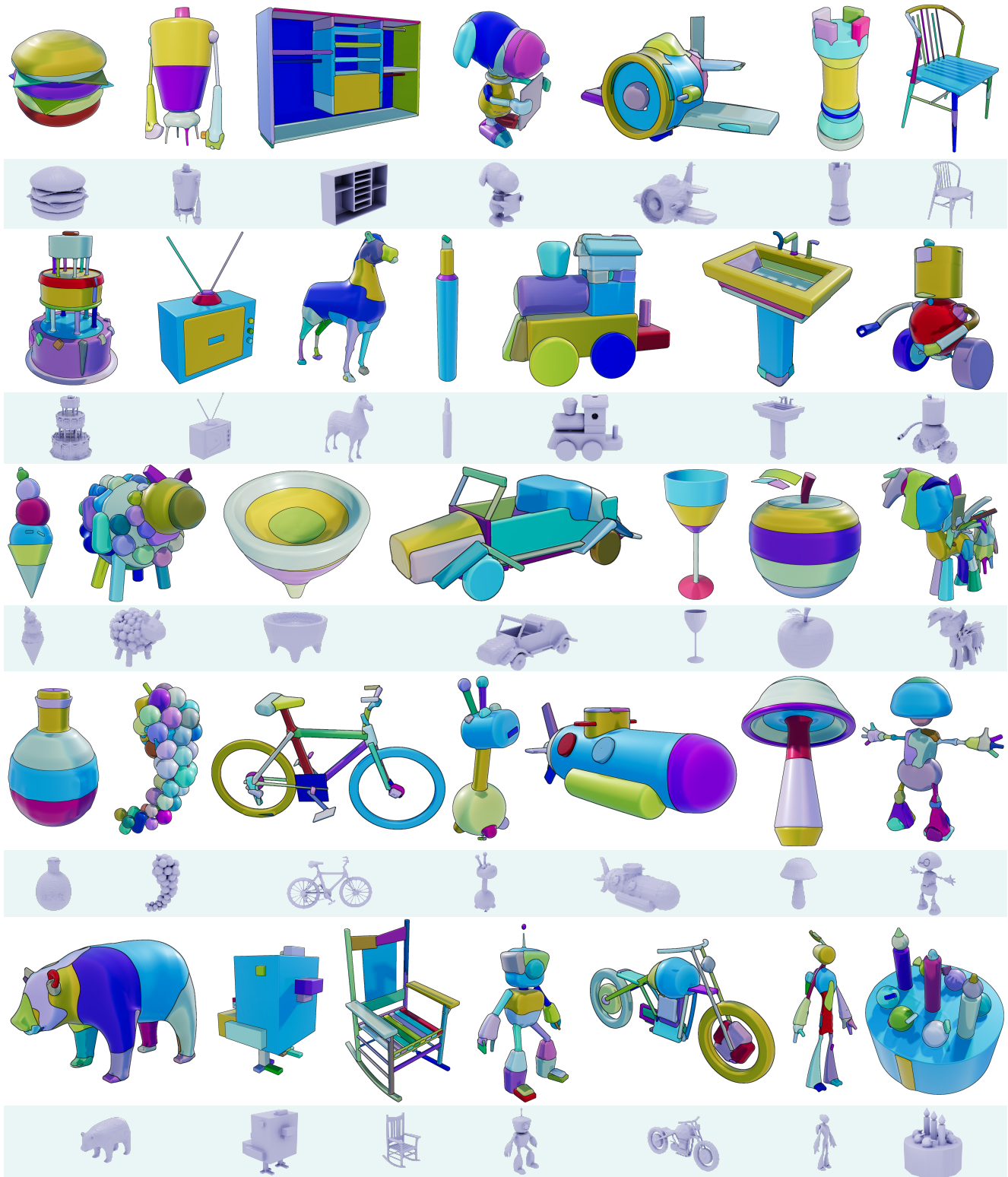
Figure 1. Qualitative results on the Toys4K dataset. Each example shows the input mesh (gray, bottom row) and the corresponding primitive assembly inferred by ResFit. These examples highlight our method’s ability to capture fine geometric detail and overall structure using compact, interpretable assemblies across a wide variety of toy categories.
