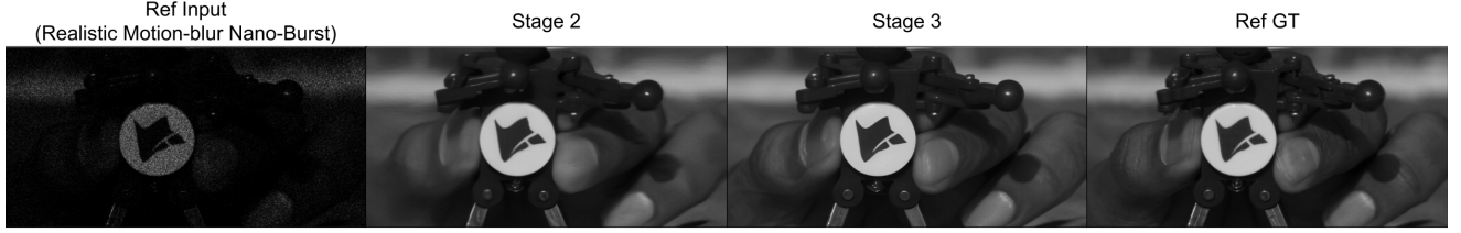
Figure 9. Stage 2 (gQIR) vs Stage 3 (Burst-gQIR) On Realistic Burst of Nano-Bursts. Motion-blur ridden nano-bursts result in Stage 2 to replicate motion blur in the output due to lack of any temporal context.
