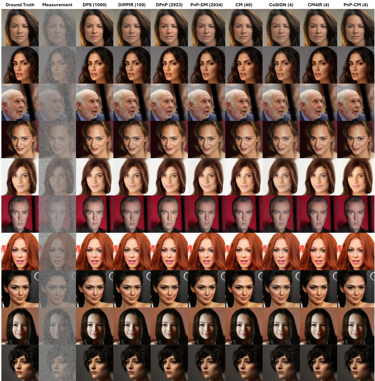
Figure 7. Demonstration of inpainting results on CelebA-HQ with \sigma_y = 0.05 . PnP-CM reconstructs the missing regions with coherent facial geometry and realistic textures, producing completions that align more closely with the ground truth than competing methods.
