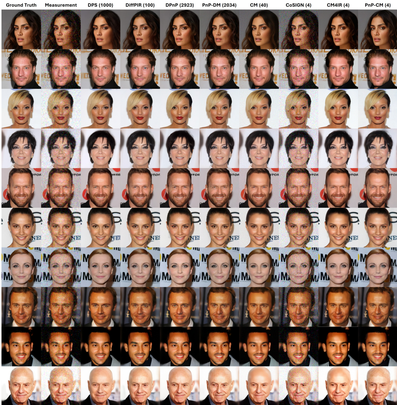
Figure 8. Illustrative 4\times super-resolution results on CelebA-HQ with \sigma_y = 0.05 . PnP-CM restores high-frequency details with improved clarity and denoising, yielding visually richer reconstructions.
