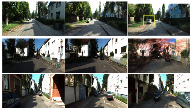
Figure 4. Qualitative results of Gen3C with cameras moving forward. Row 1 (highlighted by the yellow box) shows visual artifacts resulting from depth accumulation error. Row 2 demonstrates the abrupt degradation in scene quality, and Row 3 provides a successful example of forward scene generation.
