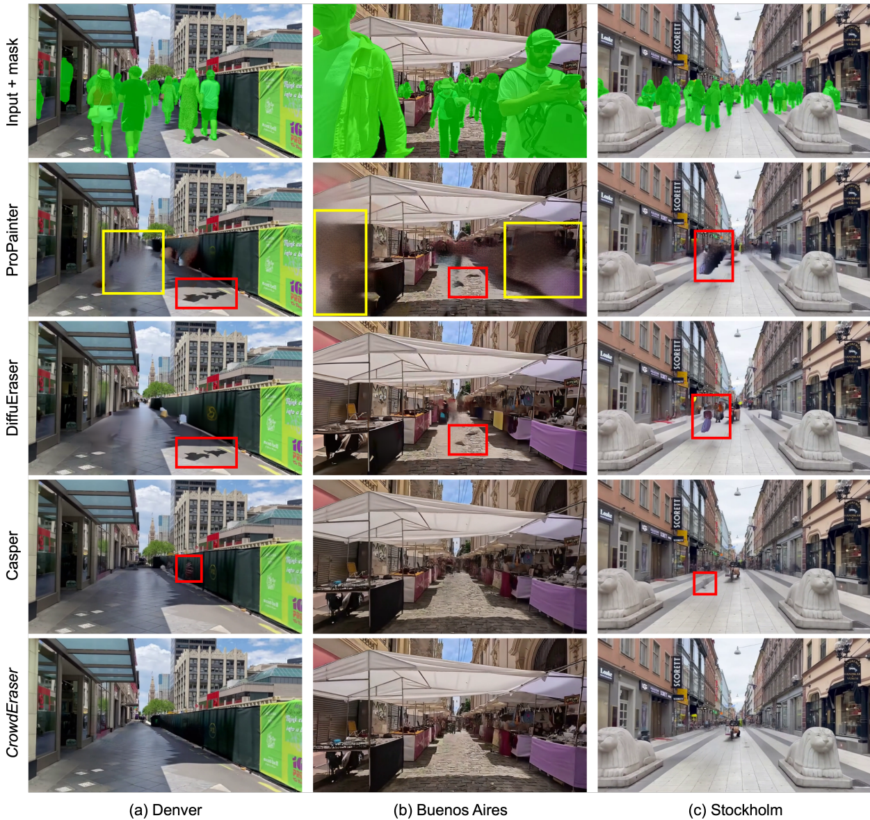
Figure 9. Full baseline comparison for the scenes in Figure 1. Red boxes indicate failures in foreground removal or shadow handling, while yellow boxes highlight blurry inpainting artifacts. ProPainter [48] and DiffuEraser [18] struggle with sharp cast shadows and often blur or lose details in large masked regions. Casper achieves more reliable effect association but exhibits noticeable hallucinations when masks become large. In contrast, CrowdEraser remains robust under significant mask sizes, preserving background structure and producing more visually plausible results.
