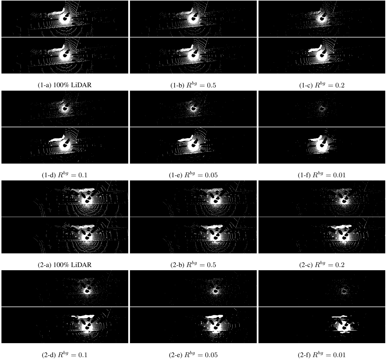
Figure 4. Pillar completion results on OPV2V. The foreground sampling ratio R^{fg}=0.2 . The top row shows the input sparse pillars under varying sampling ratios. Bottom row displays the corresponding reconstructed pillars produced by the VQ-based LiDAR completion module. 1 and 2 are different agents.
