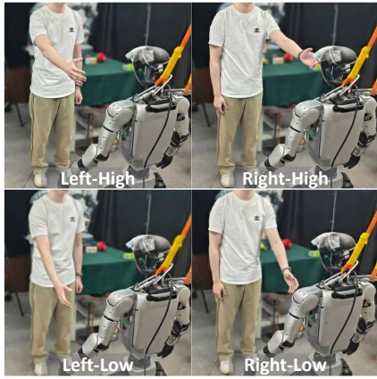
Figure S4. Counterfactual online reactivity tests on hardware. Left: handshake behavior under spatial target variations. Right: earlier or later human hand raises shift the timing of robot initiation.
