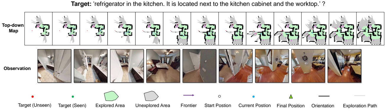
Figure 5. This visualization illustrates the process of an agent exploring and navigating to a target described by natural language—“refrigerator in the kitchen. It is located next to the kitchen cabinet and the worktop”—in an indoor environment. It is composed of three parts from top to bottom: the Top-down Map sequence, the Observation sequence (first-person visual inputs), and the legend, which respectively display the global exploration state, the agent’s local visual perception, and the meaning of each visual element.
