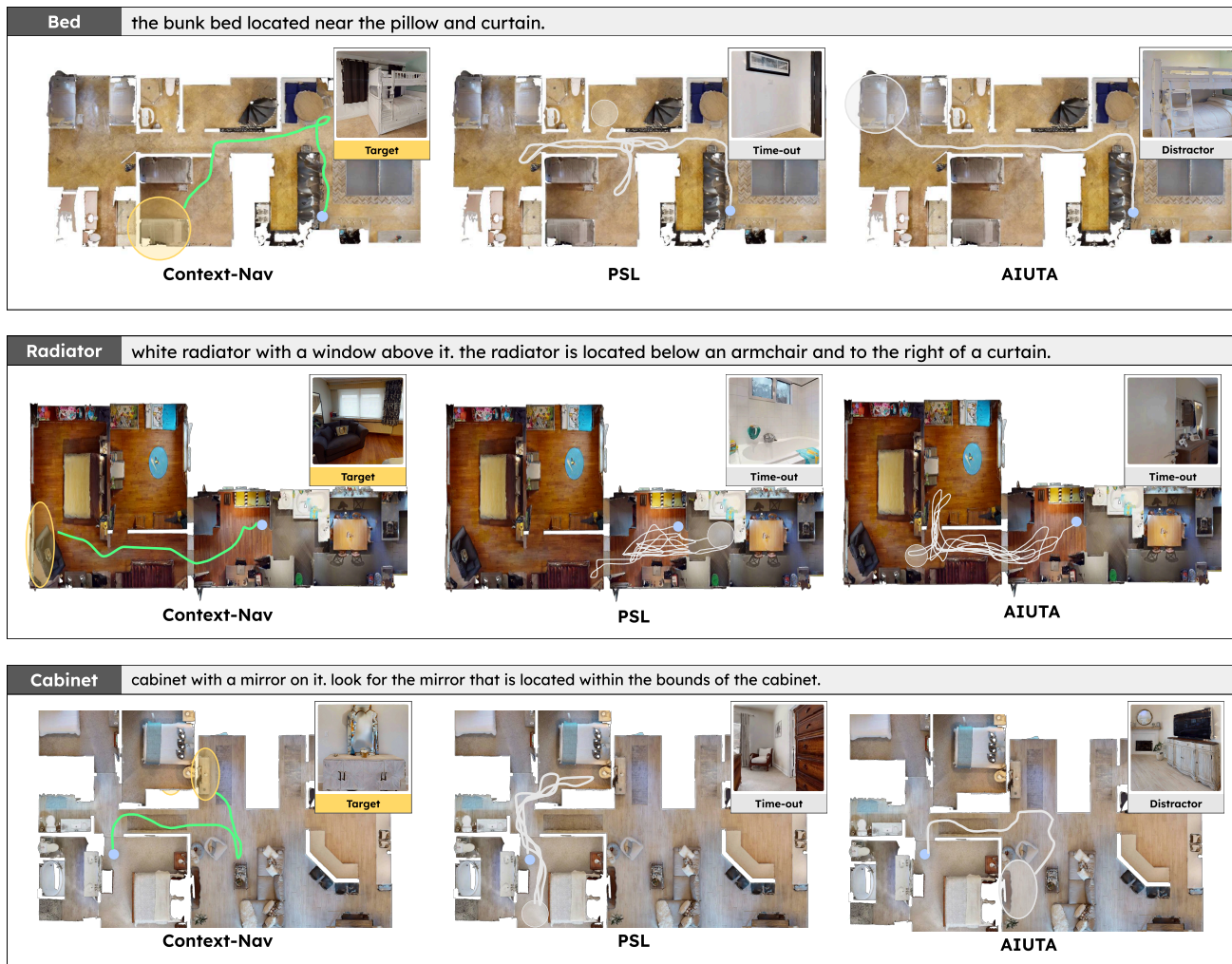
Figure S2. Qualitative comparison on CoIN-Bench. Context-Nav trajectories are compared with those of the RL-trained PSL [16] policy and the training-free AIUTA [17] agent on CoIN-Bench episodes featuring multiple same-category distractors. For each text goal, top-down trajectories are overlaid on the floor map: Context-Nav is shown in orange and the baselines in light gray. Insets show the final egocentric view and outcome label for each method: Target indicates that the correct instance is reached within the step budget, Time-out denotes failure to reach any candidate in time, and Distractor indicates that the agent stops at a different instance of the same category. In these examples, Context-Nav consistently reaches the correct instance, whereas the baselines either time out or stop at distractors.
