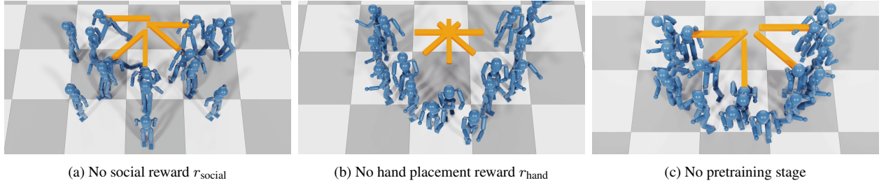
Figure S7. Simulation results obtained with variations of the final policy \pi_{\text{adapt}} under strong pushes on the back. Each still illustrates the qualitative behavior resulting from different reward configurations in the ablation study.
