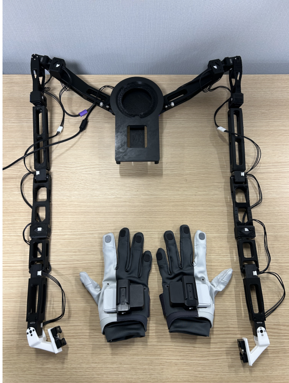
Figure 15. G1 Teleoperation System. We build the G1 upper-body teleoperation system from HOMIE [4]. We use a pair of MANUS Mocap glove to track the human hand pose.
