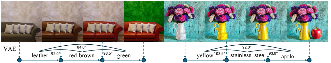
Figure 14. Editing vectors connect the VAE latent codes of different images. Angles between these vectors (derived from cosine similarity) are approximately 90^\circ , illustrating orthogonality.
