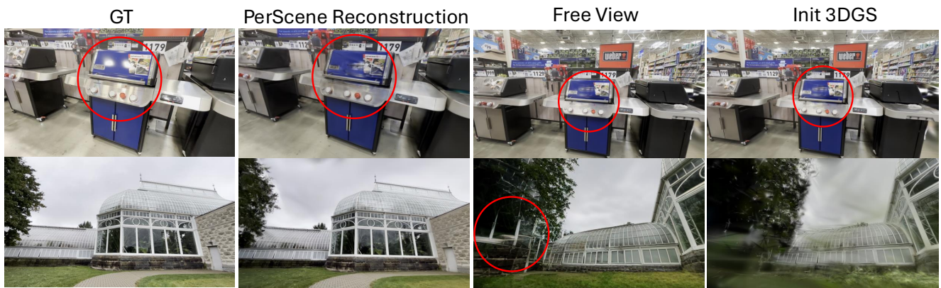
Figure 16. Failure cases of free-view generation. Red circles indicate regions where our pipeline struggles due to diffusion priors, including the incorrect handling of complex reflections (top row) and the over-sharpening of 3DGS floaters (bottom row).
