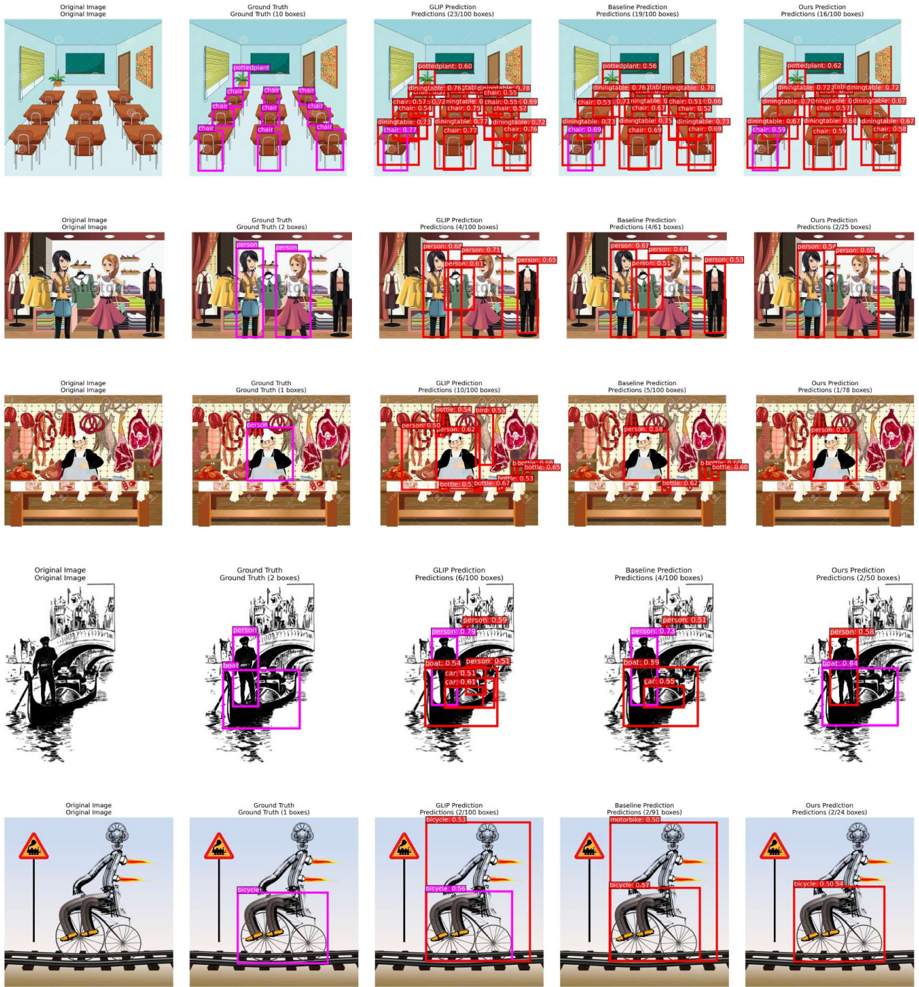
Figure 8. Comprehensive detection quality comparison across multiple test cases. Each row shows (from left to right): Original image, Ground truth annotations, GLIP predictions, Baseline predictions, and Our method predictions. Our approach consistently produces cleaner, more precise bounding boxes with significantly reduced false positives and better object-background separation across diverse scenarios and domains.
