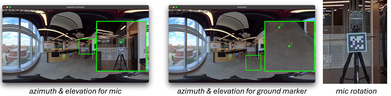
Figure 6. Calibration annotation interface. Our tool for camera–microphone calibration. Left: annotating the azimuth and elevation of the FOA microphone in the panorama. Middle: annotating azimuth and elevation for ground markers ( i.e. , the marker right below the microphone position) that define a world reference frame. Right: visualizing the relative rotation between AprilTag marker and camera, which is used to estimate the microphone orientation in the world coordinate system.
