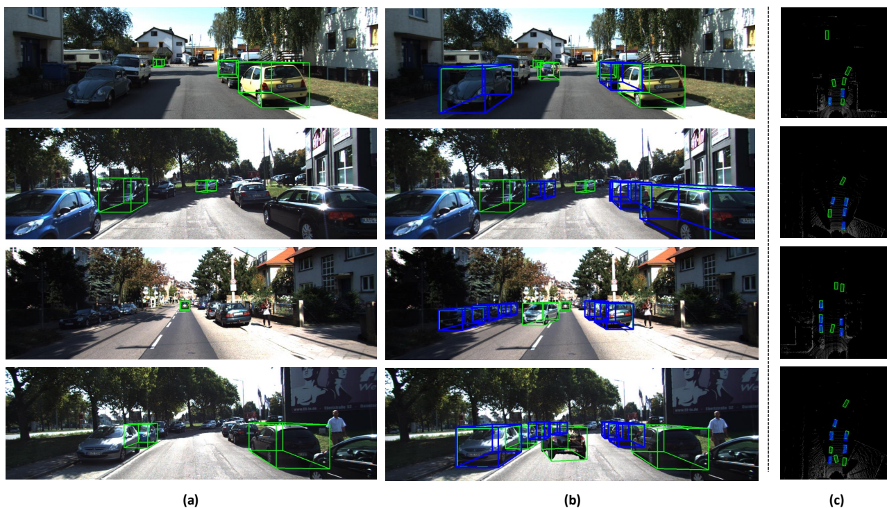
Figure S.4. Visualization of pseudo-labels added during training. (a) shows the sparsely annotated ground-truth labels. (b) presents the combined set of ground-truth and newly added pseudo-labels, where blue boxes denote the newly added pseudo-labels and green boxes represent all available labels (sparse ground-truth + accumulated pseudo-labels). (c) visualizes the BEV alignment between the newly added pseudo-labels (blue) and the original full ground-truth annotations (green), illustrating that the generated pseudo-labels are geometrically consistent with the true object locations.
