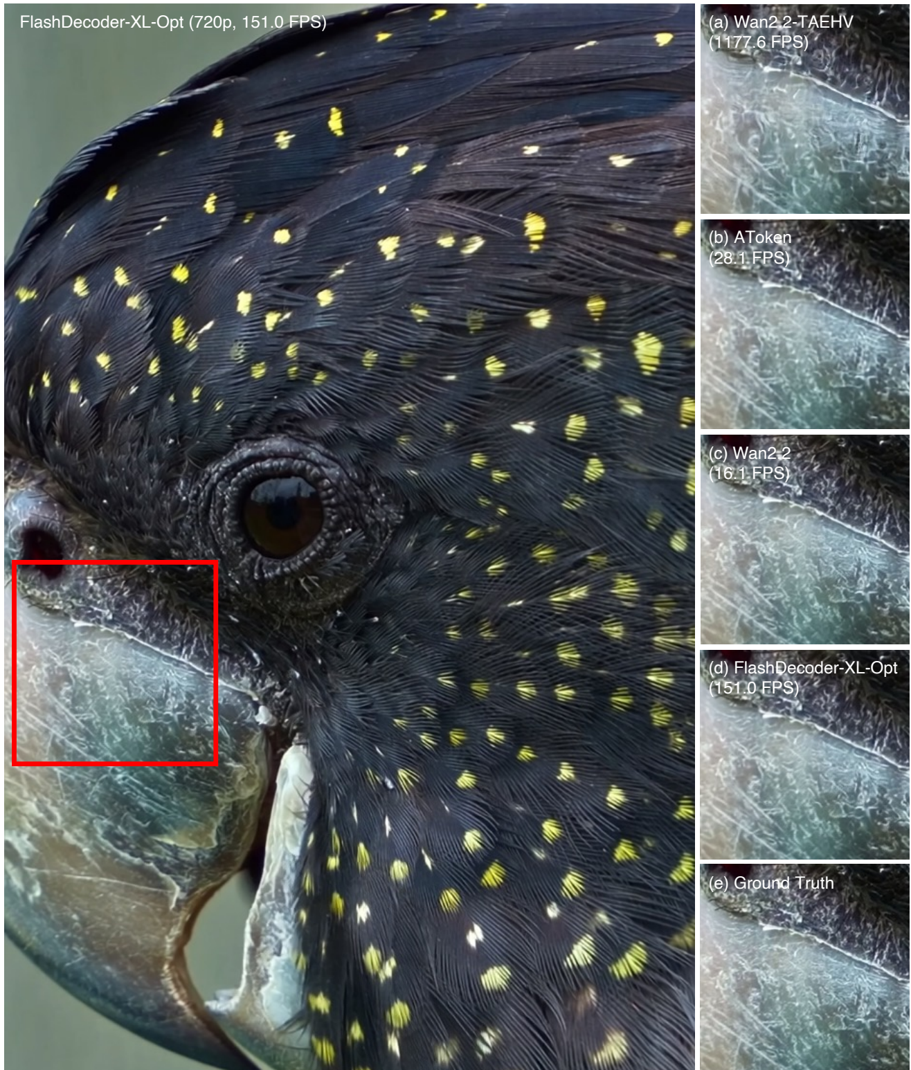
Figure A. Qualitative comparison of 720p reconstruction results. We compare reconstructed frames from video decoders with 4\times temporal and 16\times spatial compression: (a) Wan2.2-TAEHV [1], (b) AToken [13], (c) Wan2.2 [19], (d) our FlashDecoder-XL-Opt, and (e) ground truth. (a) and (b) produce blurry reconstructions, while (c) and (d) yield visually comparable outputs, yet (d) achieves over 9\times higher throughput.
