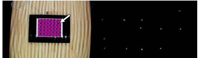
Figure 16. Overlapping pattern projected on the board (left) and an image captured by one of the embedded cameras (right).
