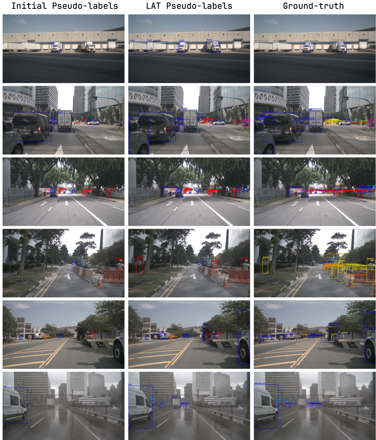
Figure 3. Qualitative results of Cityscapes target label space in class-divergent setting with nuImages dataset. Row 1: LAT recovers truck instances missing from initial pseudo-labels. Row 2: LAT refines truck bounding boxes and detects small objects. Row 3: LAT recovers heavily obscured cars. Row 4: LAT detects pedestrians omitted by upstream pseudo-labels. Row 5: LAT identifies foreground and background trucks. Row 6: LAT recovers vehicles under adverse weather conditions (rain).
