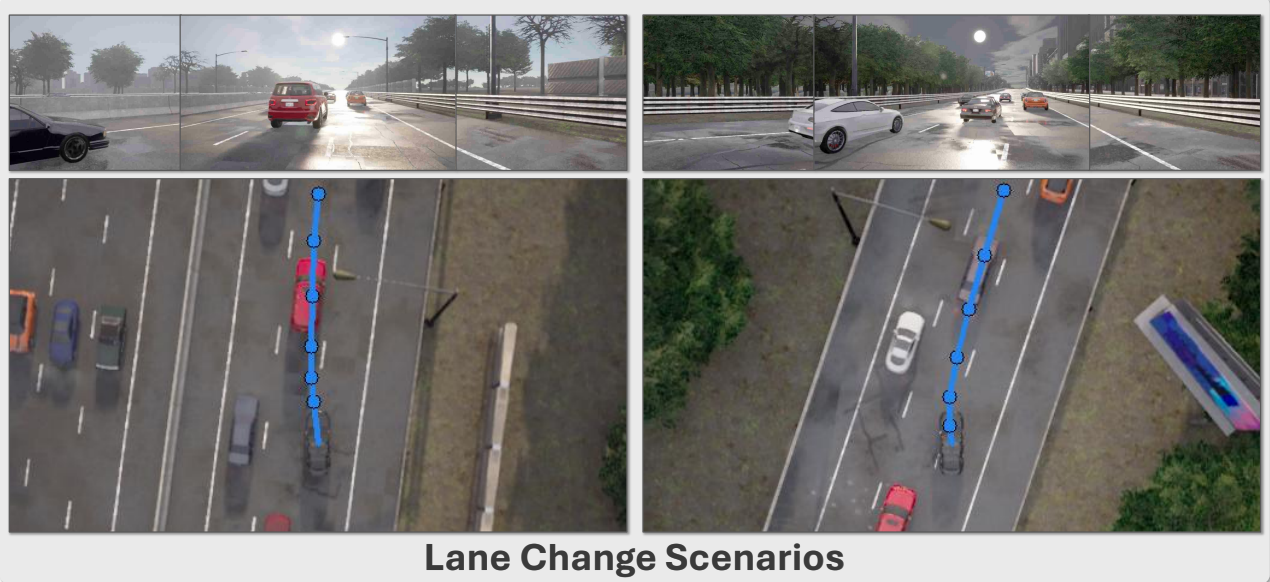
Figure 4. Visualization of the Bench2Drive benchmark. The predicted trajectories are visualized as blue curves in each scene. SafeDrive demonstrates robust performance across diverse scenarios in closed-loop environments, consistently generating stable and safe motions.
