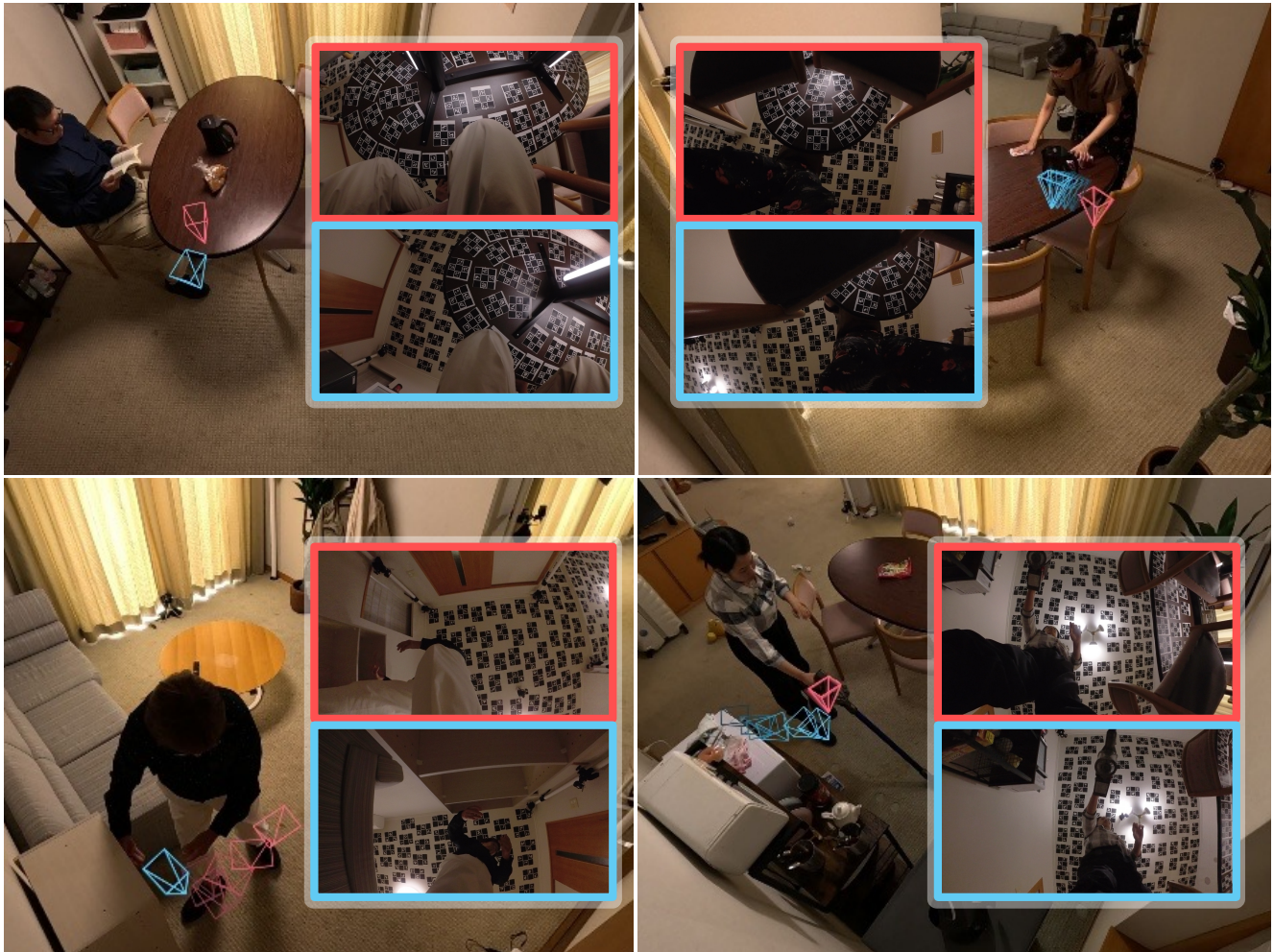
Figure E. Localized foot camera poses and the images captured from these cameras. The wide field of view of the foot cameras enables capture of many markers and accurate pose localization.
