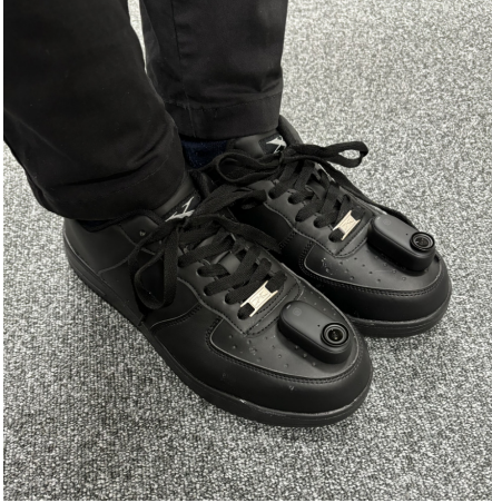
Figure B. Foot cameras attached to subjects’ feet. These cameras do not restrict the subjects’ movements and are small enough to remain invisible to the room-mounted cameras.
