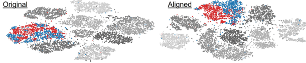
Figure 2. Test set embeddings of the DecoyMNIST MLP model before (left) and after (right) the LVLM-VA alignment step. The clusters are more separated, as the model is less affected by spurious shortcuts.
