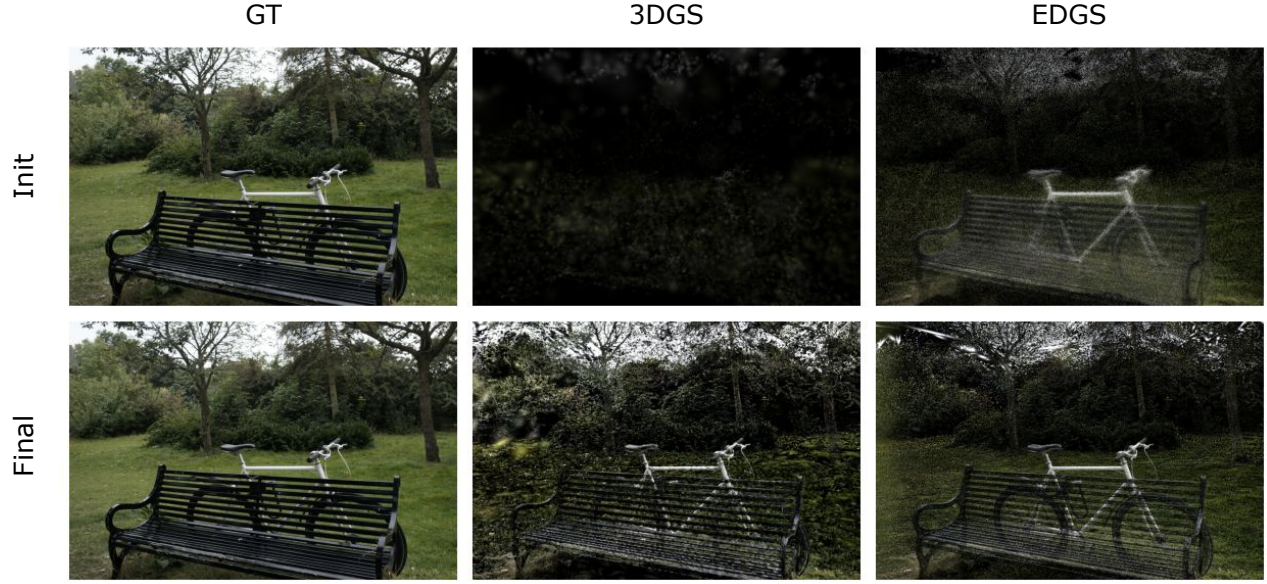
Figure A2. Reduced-scale splat renderings from training views. We visualize the initialized and converged splats of baseline 3DGS and EDGS using the standard Gaussian renderer while reducing splat scales so that individual Gaussians become visible. EDGS already initializes the scene with the splats required for the final reconstruction, whereas baseline 3DGS starts from a much coarser scaffold and only reaches a similar distribution after optimization and densification. This highlights that EDGS begins near the converged spatial distribution that standard 3DGS must discover iteratively.
