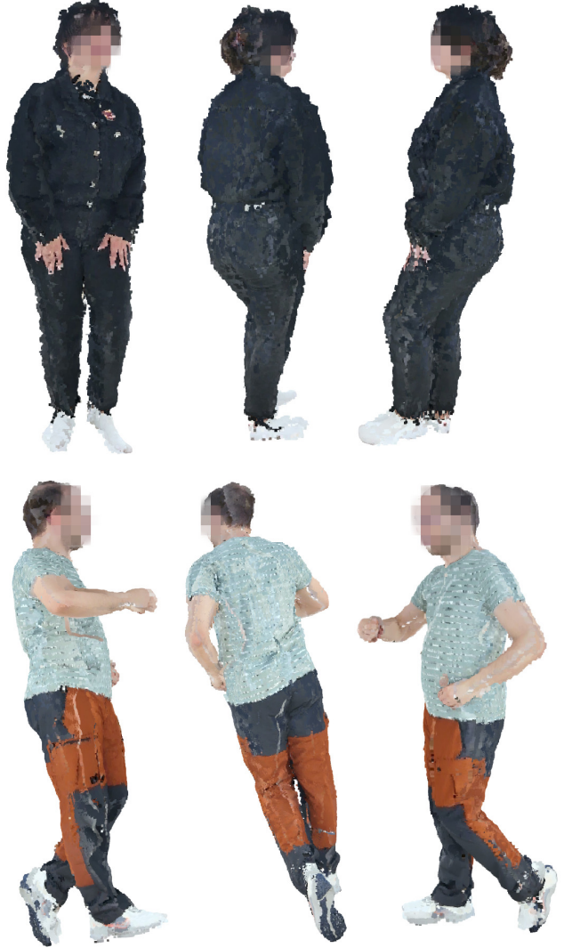
Figure 10. Examples of the reconstructed point clouds visualized from different viewpoints. We apply no post-processing on the point clouds, including 3D and color smoothing. We preprocess the depth images to filter the boundary noise by masking out the pixels that have an absolute difference above 15 mm with their nearby pixels.
