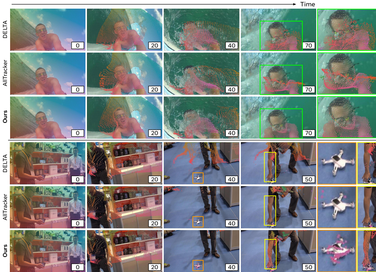
Figure 10. Qualitative comparison on challenging sequences involving non-rigid water motion and small object tracking. Columns compare DELTA, AllTracker, and Ours. The top sequence exhibits large non-rigid motion and drastic appearance changes as the person dives into the water. The bottom sequence features large camera motion where objects repeatedly go out of frame, requiring the tracking of a small object. Our method maintains a consistent track in these difficult conditions, whereas DELTA and AllTracker fail to recover or exhibit drift. Notably, our approach successfully tracks the small object in the bottom sequence, thanks to our high-resolution feature maps that preserve fine details. Numbers in lower-right boxes indicate frame numbers.
