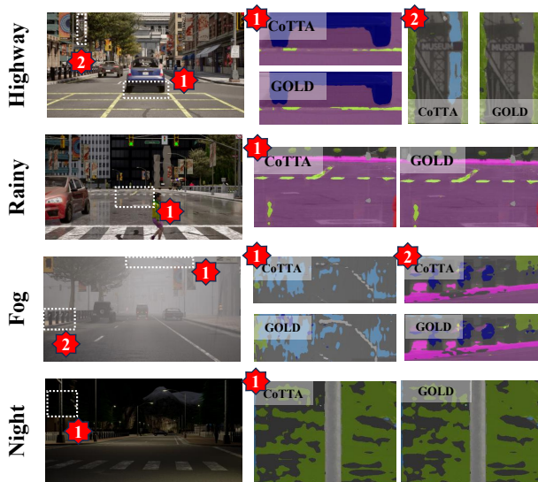
Figure S2. Detailed segmentation comparisons (cropped views). White boxes indicate regions shown at higher resolution to emphasize the qualitative gains of GOLD in challenging conditions (shadows, reflections, fog/night).
