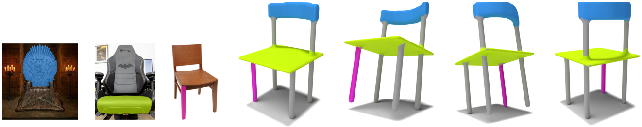
Figure 16. A single view to a complete 3D part. Although each image depicts only one view of the object (left), the entire corresponding part is successfully segmented in 3D (right).
