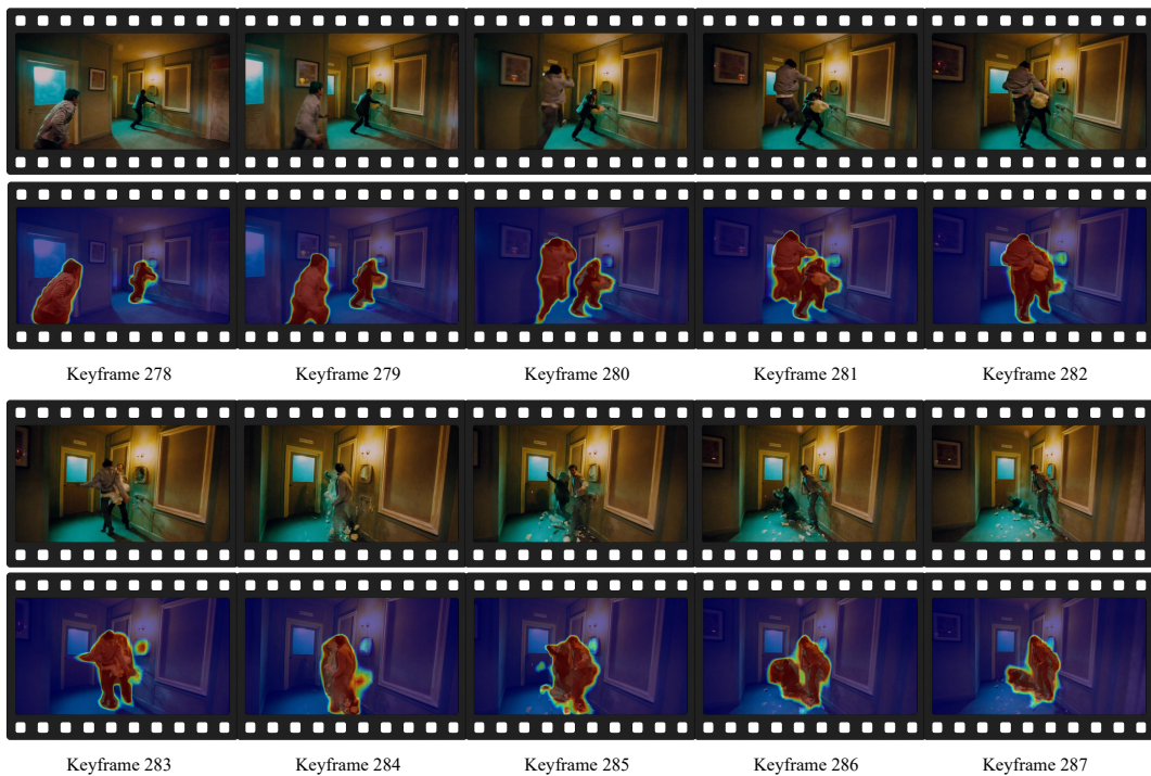
Figure 7. Uncertainty Visualization for Consecutive Frames of YouTube Tomyum 2. Our approach assigns high uncertainty to regions exhibiting strong view-dependent effects (e.g., the mirror).
