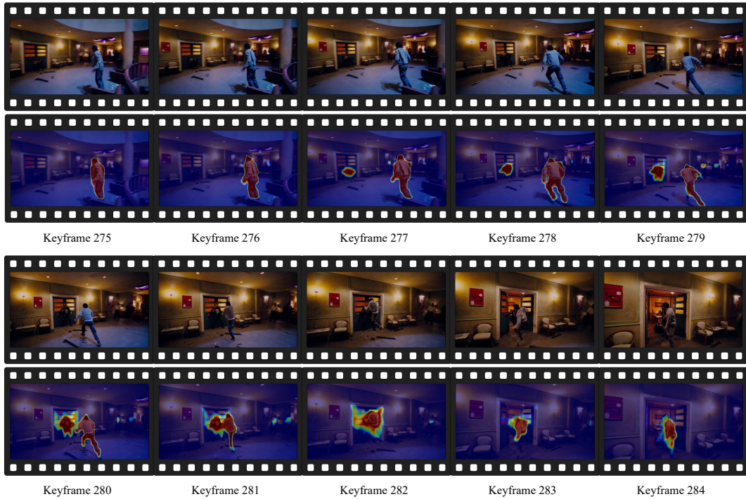
Figure 6. Uncertainty Visualization for Consecutive Frames of YouTube Tomyum 1. We observe that our method robustly handles scenarios in which an object transitions from a static state to dynamic motion, such as a door being pushed open by a person. Prior to the onset of motion, our approach leverages stable visual correspondences on the door to help tracking, since our uncertainty optimization is based on frame-to-frame feature alignment.
