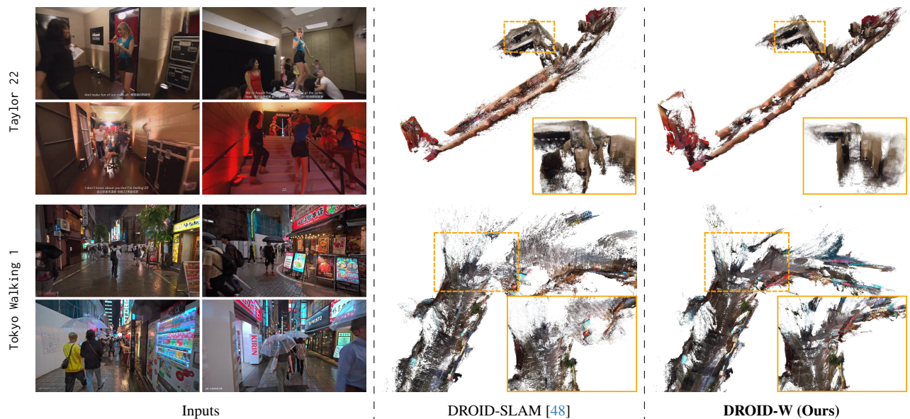
Figure 8. 3D Reconstruction Comparisons on YouTube Sequences. We compare reconstructed static point clouds between DROID-SLAM [48] and our method. Our approach produces more accurate and consistent reconstructions across highly dynamic and visually challenging real-world sequences. For the Taylor 22 scene, DROID-SLAM reconstructs two separate corridor structures due to inaccurate pose tracking, as highlighted in the boxed region, whereas our method produces a consistent geometric reconstruction. Moreover, the white lane marking on the asphalt road of Tokyo Walking 1 is faint and fragmented in the point cloud reconstructed by DROID-SLAM, while in our reconstruction it remains cleanly visible, continuous, and highly accurate.
