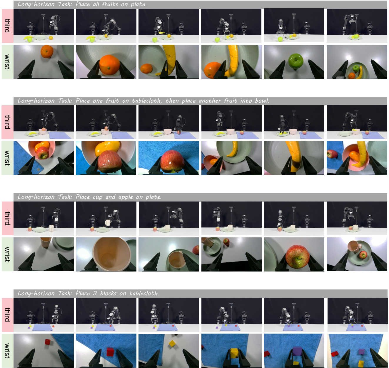
Figure 2. Qualitative results of OptimusVLA on Real-World. From top to bottom, we illustrate four Long-horizon Tasks : Place all fruits on plate , Place one fruit on tablecloth, then place another fruit into bowl , Place cup and apple on plate , and Place 3 blocks on tablecloth . Here, third denotes third-person view images, while wrist denotes images captured from the robot’s wrist-mounted camera.
