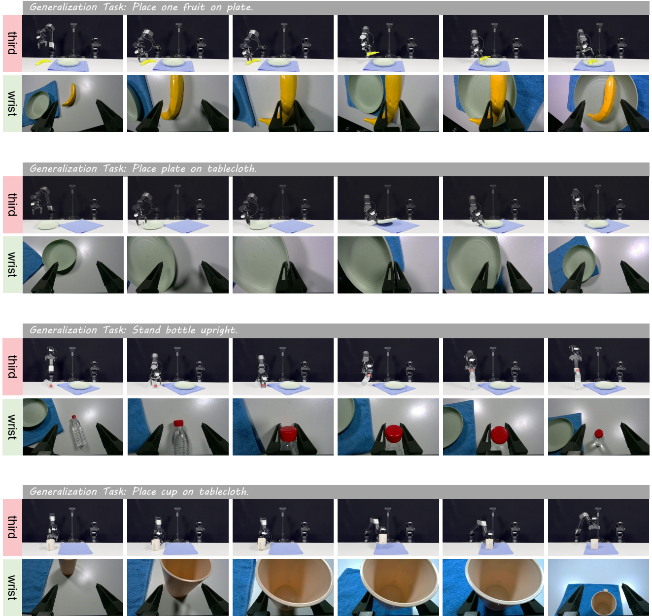
Figure 1. Qualitative results of OptimusVLA on Real-World. From top to bottom, we illustrate four Generalization Tasks : Place one fruit on plate , Place plate on tablecloth , Stand bottle upright , and Place cup on tablecloth . Here, third denotes third-person view images, while wrist denotes images captured from the robot’s wrist-mounted camera.
