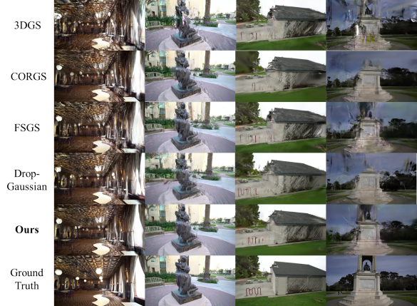
Figure 7. Qualitative Comparison on Tanks for 3 training views. In large-scale dataset, 3DGS and DropGaussian struggles to maintain geometry and texture fidelity, exhibiting significant artifacts. FSGS and CoR-GS recover coarse structure yet still exhibit over-smoothed geometry and artifacts. In contrast, HeroGS reconstruct fine structures and high-frequency textures.
