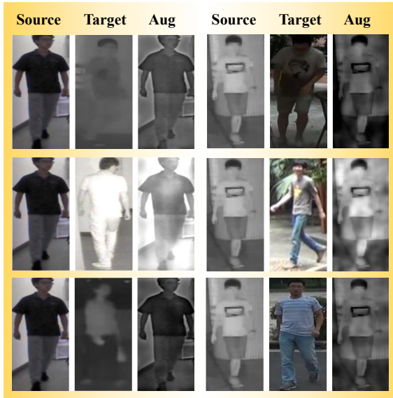
Figure 2. Visualization of Random Frequency Augmentation. The enhanced image (Aug) is obtained by exchanging the low-frequency amplitudes of the source image with the target image.
