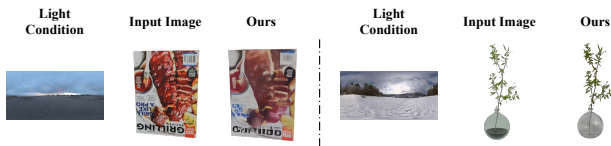
Figure 13. Failure Cases. Left: High-frequency details (e.g., text) are blurred due to voxel resolution constraints and VAE compression loss. Right: Transparent objects exhibit checkerboard artifacts. While 3DGS theoretically supports alpha blending, data scarcity in current datasets leads to inaccurate density estimation for refractive surfaces.
