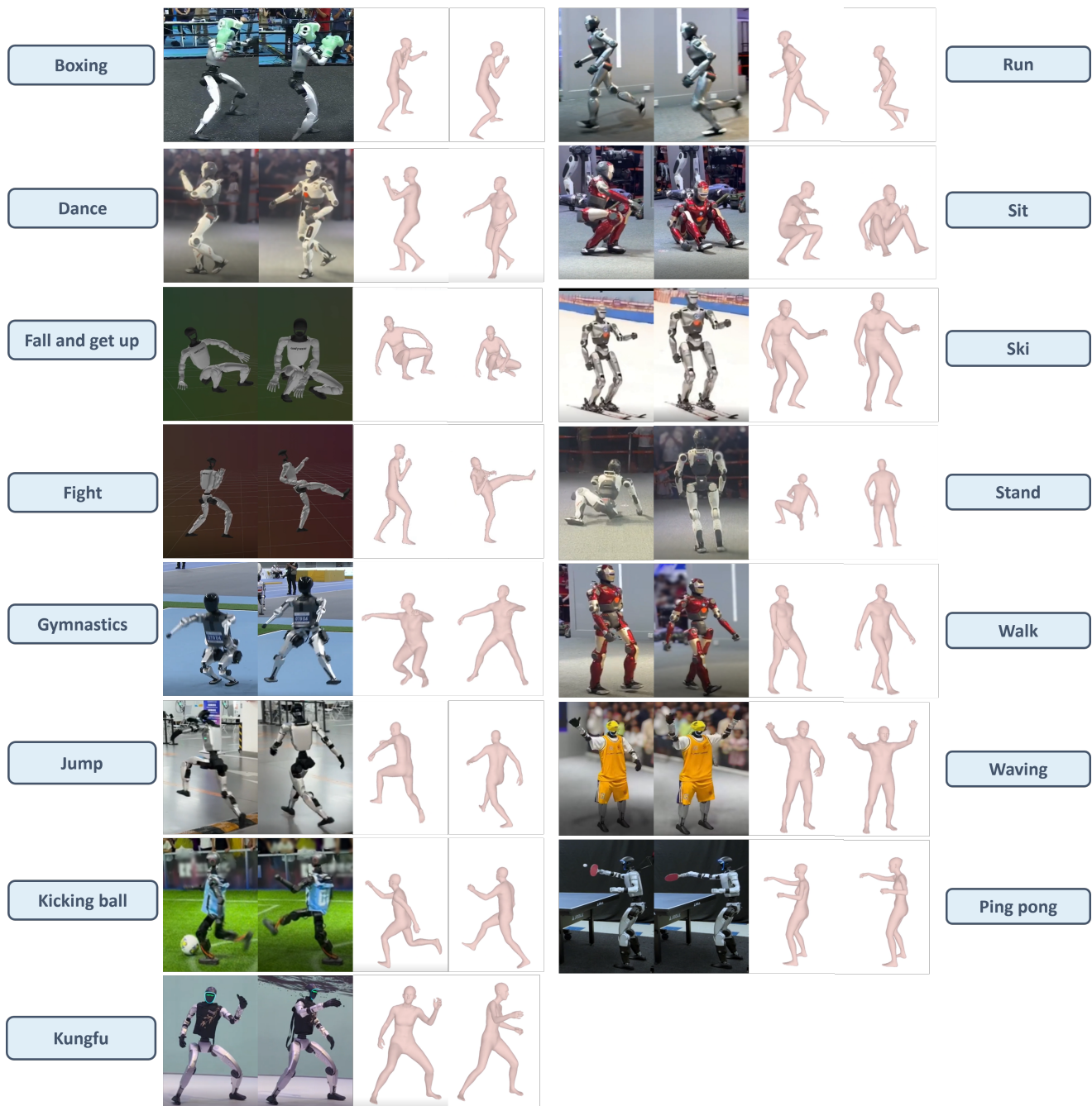
Figure S8. Fifteen humanoid motion categories. This figure illustrates the full set of 15 action categories captured from real-world and simulated humanoid robots in HHMotion, covering both sport and daily motions.
