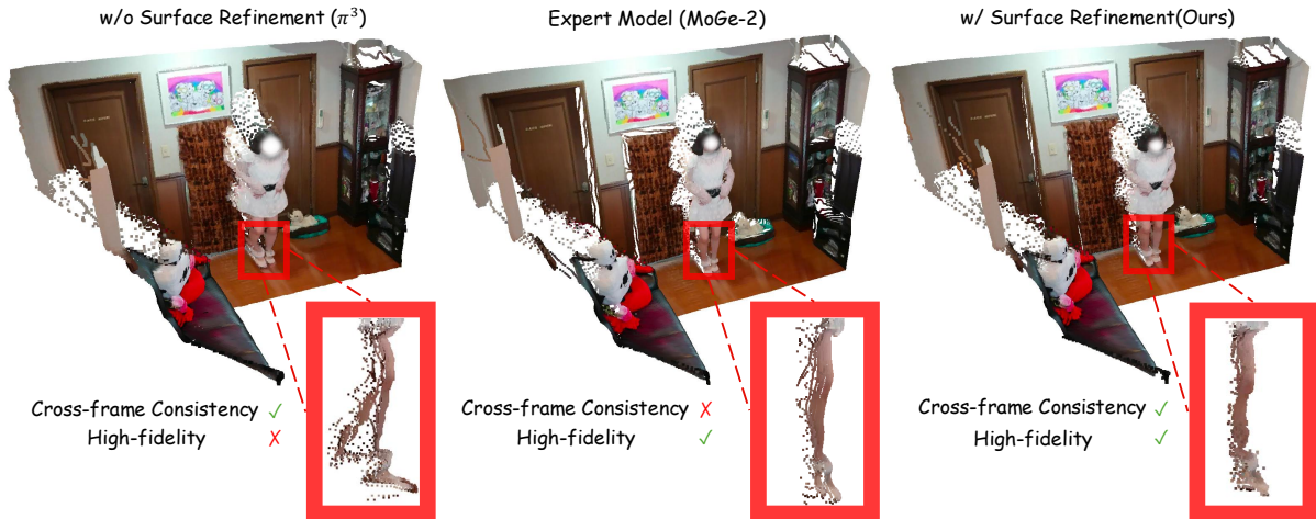
Figure 6. Qualitative Impact of Human Surface Refinement. Comparison illustrating the effectiveness of our specialized surface refinement strategy. The \pi^3 baseline (Left) provides good cross-frame consistency but the reconstructed human geometry is coarse and does not conform well to the body shape. The Expert Monocular Model (MoGe-2) (Center) achieves high fidelity but lacks multi-view consistency. Our full method (Right) successfully distills the high-frequency surface details into the multi-view reconstruction framework, achieving both high fidelity and strong cross-frame consistency.
