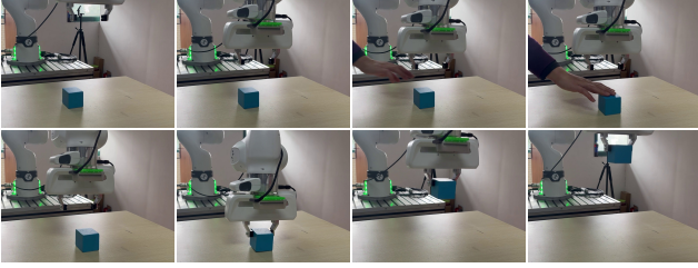
Figure 8. Dynamic objects. FLA successfully adjusts trajectories in real-time against manual target disturbances.
