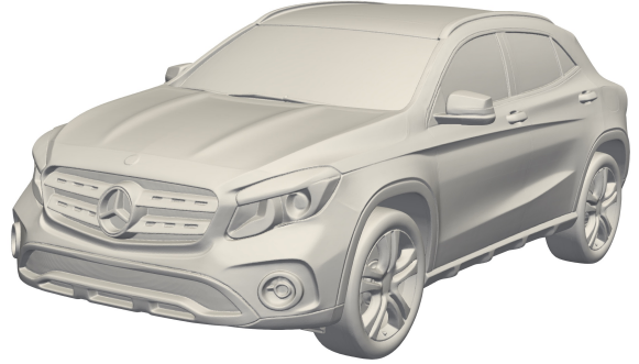
Figure 17. Effect of prompt normalization on 2D conditioning images. Top: without prompt normalization, the same text prompt often produces images with turned wheels and additional non-body structures (for example floor plates and artefacts under the sills), which lead to three-dimensional meshes that are unsuitable for CFD. Bottom: with prompt normalization, the generator produces a neutral studio view with straight wheels and no extra structures, resulting in a clean, CFD-ready mesh.
