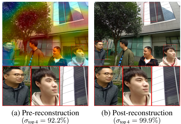
Figure S6. Comparison of results before and after low-rank prior reconstruction. Here, \sigma_{\text{top } 4} denotes the total energy of the correction flow captured by the top 4 singular values. (a) The initial correction result and confidence map. Low-confidence regions (blue masks) are magnified for a better view. (b) The post-reconstruction result.
