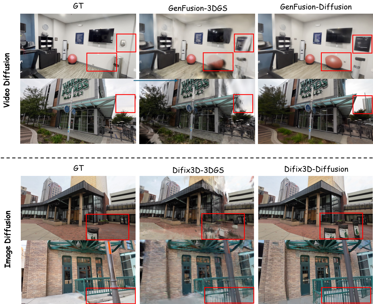
Figure 4. Qualitative demonstration of hallucination patterns in diffusion-assisted 3DGS pipelines. Both Difix3D (image diffusion) and GenFusion (video diffusion) iteratively enhance the 3DGS rendering. As a result, even mild artifacts in the initial 3DGS output, such as small floaters or subtle geometric distortions, can be progressively amplified by diffusion priors and eventually evolve into clearly visible hallucinations. This demonstrates that hallucination is not introduced abruptly, but can accumulate and become more pronounced during iterative refinement. Note: method-3DGS denotes direct rendering from 3DGS, while method-diffusion denotes diffusion-enhanced results.
