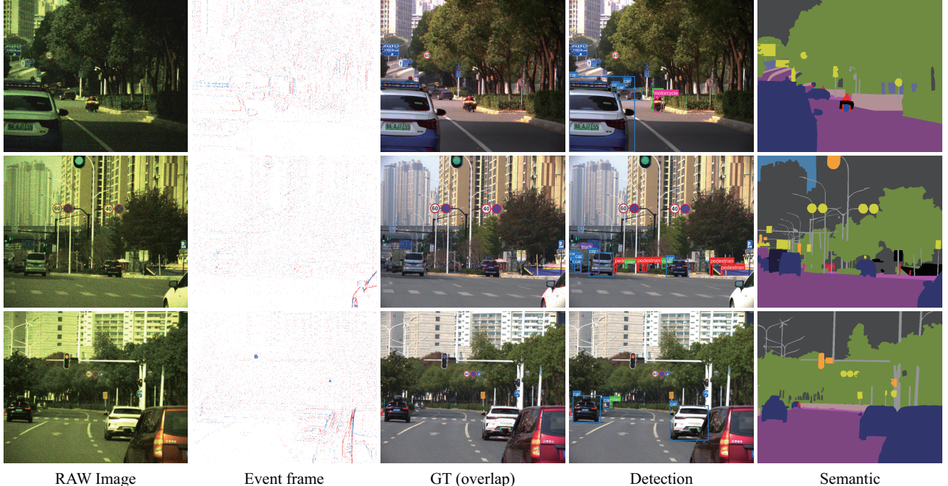
Figure 1. Visualization examples from the REAL dataset. From left to right: linearly brightened RAW images, event frames, overlays of events and ground truth (GT), object detection annotations, and semantic segmentation annotations.
